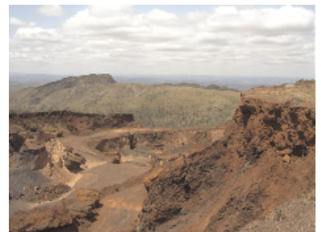
Partial view of an opencast iron-ore mine, showing the superficial crust removal.
